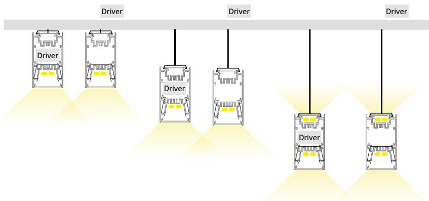
Extrusion can be surface mounted to ceilings with brackets or suspended using suspension kits.
