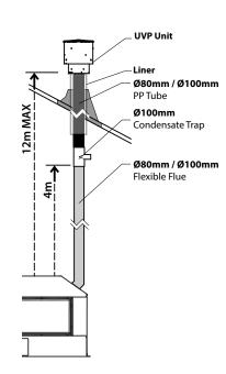
**Vertically Terminated Externally:** (utilizes the escea external vertical power flue enclosure kit)
