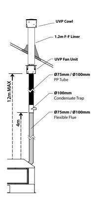
**Vertically Terminated Internally:** (utilizes the escea internal vertical power flue enclosure kit)
