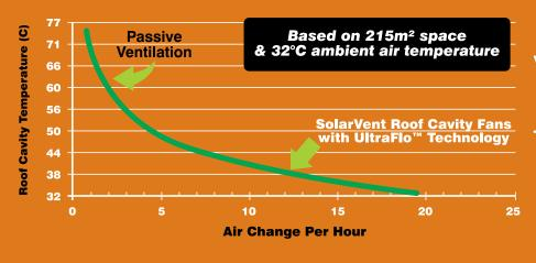
EFFECT OF VENTILATION ON ROOF CAVITY TEMPERATURE
