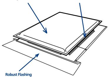
The Tile Skydome™ model features a Direct Flow System. This water removal system is an integral section located on both sides of the flashing. It provides a primary and secondary watercourse for an absolutely watertight installation and aids self-cleaning.
