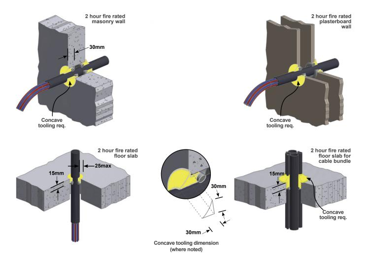
\*NOTE: Fireban One is to be filled to depth of plasterboard in one hour systems.
