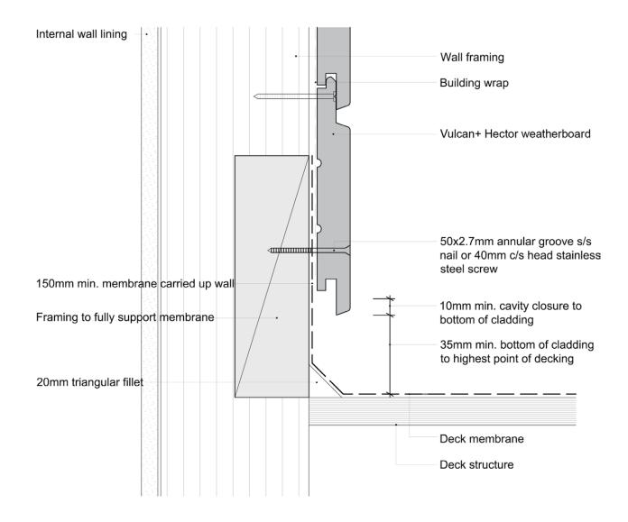
Enclosed Deck - Timber Substrate, Direct Fix
