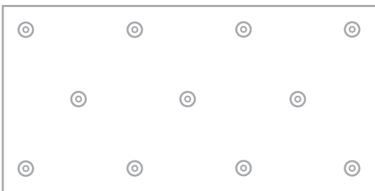
Figure 3 Fastener pattern (11 No. per board) Board size to 2400 mm x 1200 mm - 3.81 fixings / m 2
