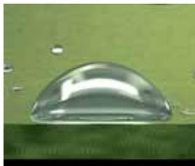
The relatively smooth cellular structure of standard webbing allows the water drop or dirt to adhere to the surface, allowing for the ingress of water into the webbing through wicking.
