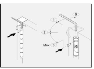
Multiple adjustment points for increasing or decreasing the spring's tension. Simple function, pull pin, turn head with allen key and replace pin. No need to remove door
