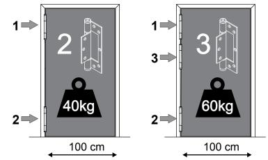
Based on a sliding scale, typical number of hinges per door start at 2 for all doors that are 1000 mm wide at or below 40 Kg. Doors around the same width but weigh from 40Kg up to 60Kg typically require 3 hinges. Note: 2nd hinge sits 5cm under the 1st hinge if 3 hinges are being used.
