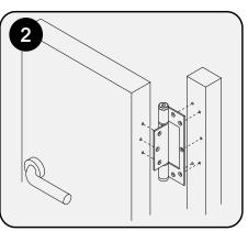
Easy 2 step installation process. Step 1, insert allen key into head and turn to set tension reinsert pin. Step 2, screw or rivet hinge to door and door jam. Easy. You're done.
