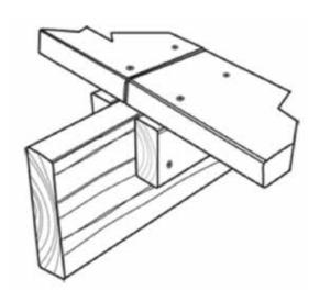
Pre-drill and countersink all deck screws, regardless of type, that are within 75mm of the end of the deck board.
