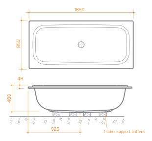
On the indicator lines, position and fix timber supports to base of the bath and floor with an approved floor and wall panelling adhesive or equivalent adhesive to provide a neat fit support. Ensure the rim of the bath is levelled during this procedure.
