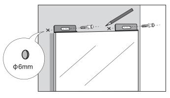
The glassless mirror can be moved backwards and forwards slightly in L-shaped brackets, and the left and right glassless mirrors are adjusted to the same line, then tighten the self-tapping screws.
