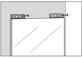
According to the position of the L-shaped bracket installed at the four corners of the mirror, fixing the φ 6mm holes position on the wall, and placing the expansion tube into it.
