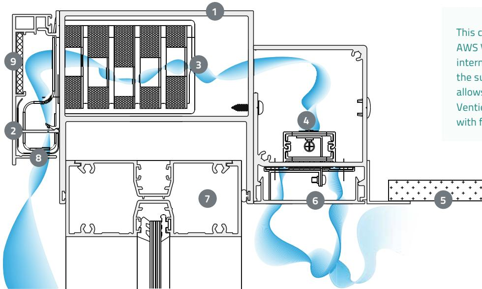
This configuration shows the AWS Ventient™ housed within an internally mounted box fixed to the sub-head. This configuration allows access to the AWS Ventient™ device when installed with flush plasterboard ceilings.
