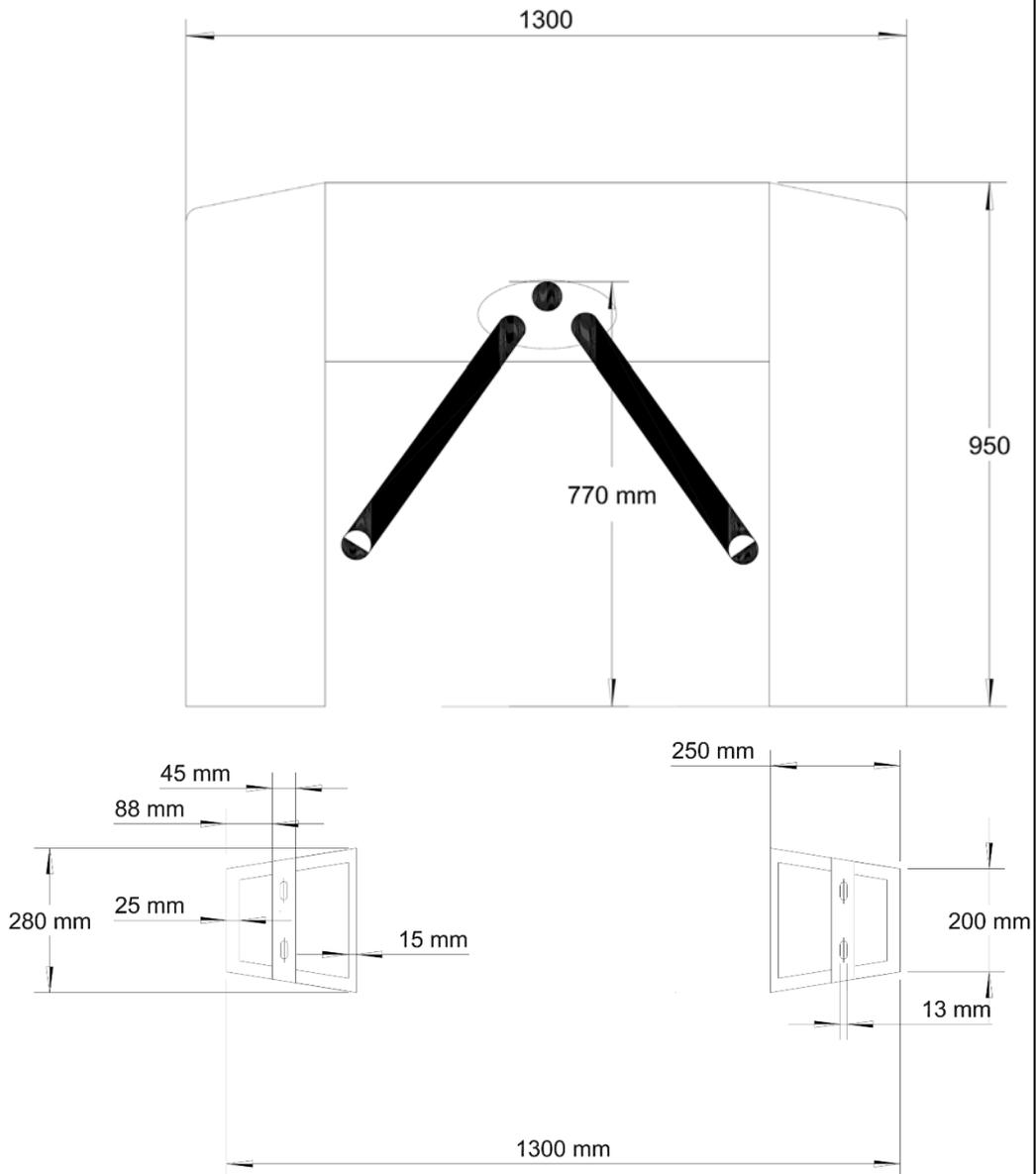
**NOTE:** The concrete pad should be 20Mpa (min) 150 mm thick, cured for 7 days on a suitably compacted foundation. Hold down anchors (4) to be 12mm dia x 100mm into the concrete.
