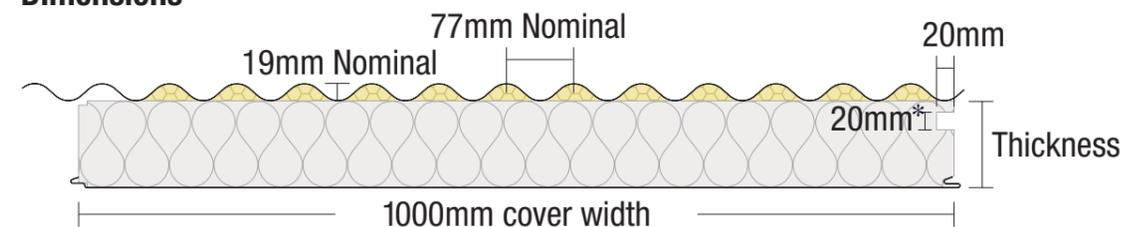
\* Services ducts 30x30mm are available for panel thicknesses 150-200mm.
