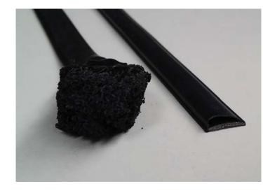
Right image: shows LAS1602BB seal before and after exposure to elevated temperature
