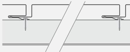
*Interlocking cassette panel profile and installation shown on top hat beam.*
