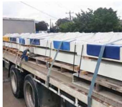
Products must be properly secured with edges protected during transportation.
