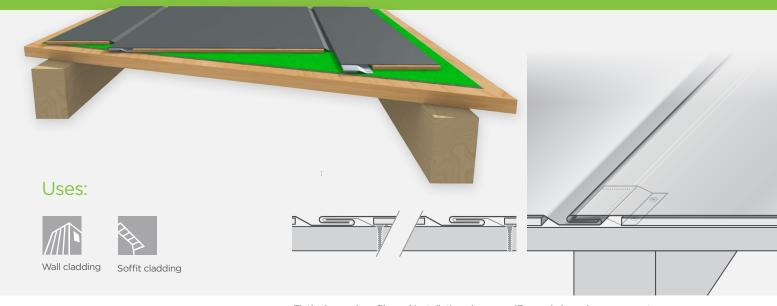
Flatlock panel profile and installation shown on 17mm ply board over supports.
