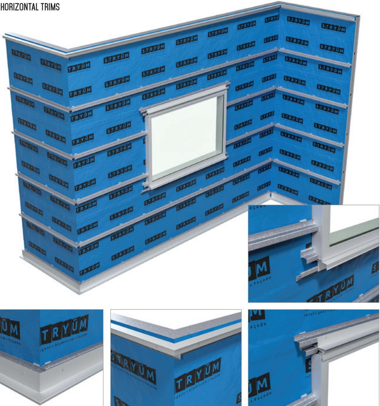
Install the horizontal trims for the cladding, at the top and bottom of the cladding section, above and below any wall penetrations, and at any slab junctions. When installing down to an adjacent flat surface such as a garden bed or pathway, a minimum of 150mm from the ground is recommended to prevent rain splash back dirtying the façade.
