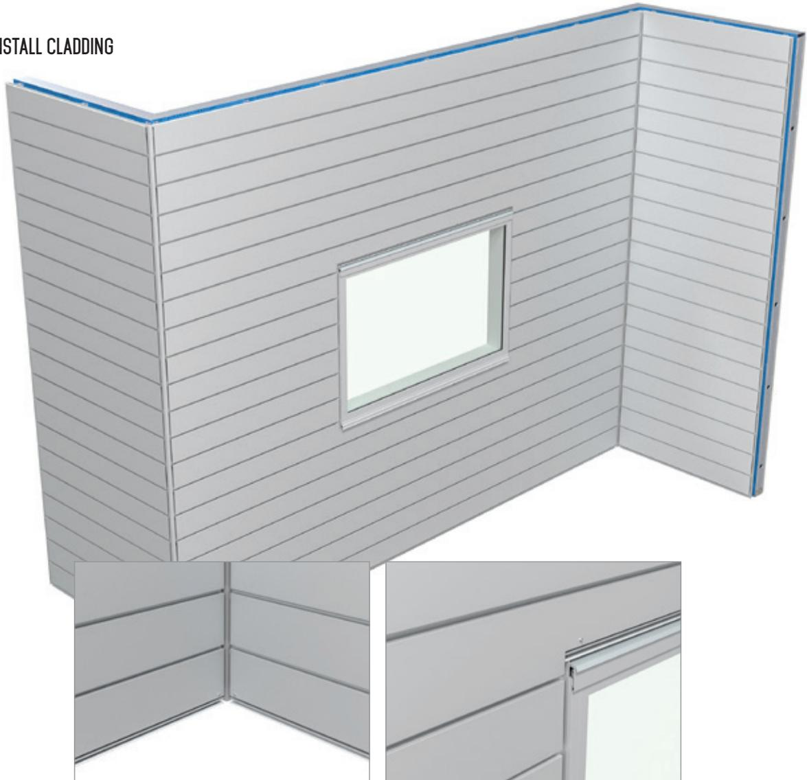
Install the cladding by cutting the panels to length, hooking the panel into the previous panel, and affixing to the S Batten. Due to the rainscreen façade system Stryüm utilizes, a minimum airflow gap of 10mm must be maintained at the top and bottom of the cavity.
