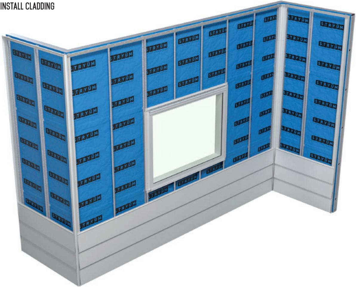
Install the cladding by cutting the panels to length, hooking the panel into the previous panel, and affixing to the S Batten. Due to the rainscreen façade system Stryüm utilizes, a minimum airflow gap of 10mm must be maintained at the top and bottom of the cavity.
