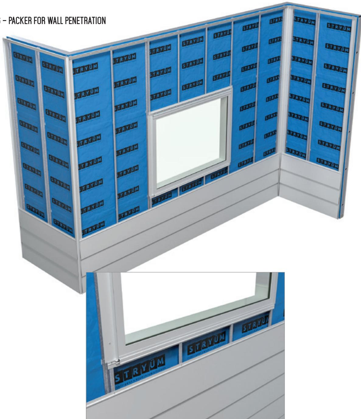
Due to the sloping nature of Step, the depth packer required to support the panel around wall penetrations will depend on where the penetrations sit down the panel. Measure carefully where the panel needs to be cut, and calculate the packer required before.
