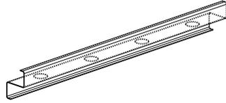
Use Stryüm Perforated S Batten as the top most batten.
