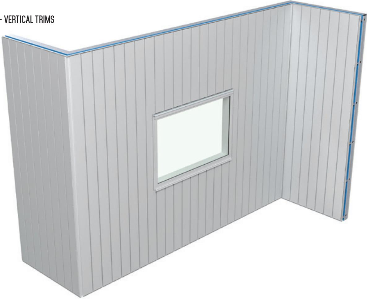
Install the cladding by cutting the panels to length, hooking the panel into the previous panel, and affixing to the S Batten. In this diagram the cladding direction chosen is Left-Right.
