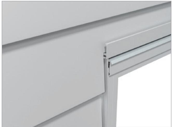
Install the cover sections to the two-piece trims to conceal rivets and cut edges. Push firmly into place, a rubber mallet may be used paying careful attention to the finish.
