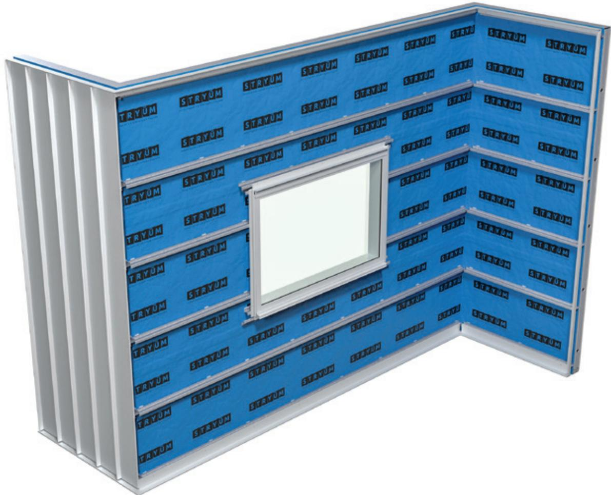
Install the cladding by cutting the panels to length, hooking the panel into the previous panel, and affixing to the S Batten. In this diagram the cladding direction chosen is Left-Right. Due to the rainscreen façade system Stryum utilizes, a minimum airflow gap of 10mm must be maintained at the top and bottom of the cavity.
