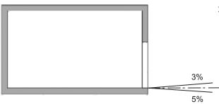
The illustrated maximum approach angles must not be exceeded. Incorrect approach angles will cause serious maneouvring positioning problems on the parking system for which the local of LevantaPARK accepts no responsibility.
