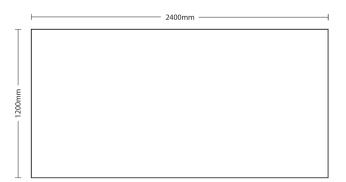
For example: A floor to ceiling panel with 2400mm ceiling height can utilise the full panel height. However above a storage unit the required height would be less, and the off-cut could be used above a door opening.
