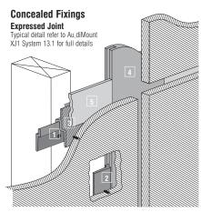
Expressed Joint - Plan view Au.diMount Concealed Fixing System (Refer to Installation System - XJ1)
