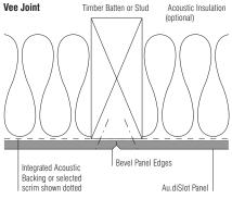
\*Vee jointing may create difficulties with panel and perforation alignment
