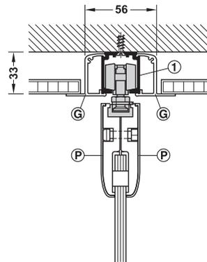
Ceiling installation with running track and 2 x clip panel for integration in suspended ceilings
