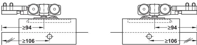
Version **A1** & **A2** Without soft and self closing mechanism
