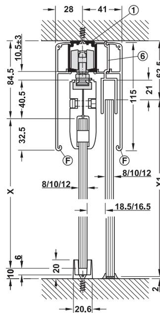
Ceiling installation with running track and clip panel 115 mm including fixed component on wooden supports (wet sealed) provided on site
