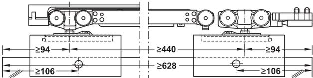
Version **B1** & **B2** With soft and self closing mechanism on one side
