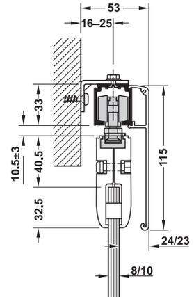
Wall mounting with clip panel and concealed mounting bracket
