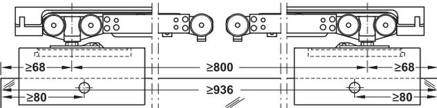
Version **E1** & **E2** With soft and self closing mechanism on both sides (2 x one-sided)
