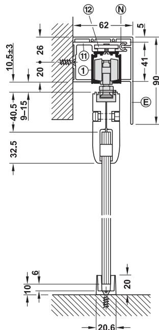
Wall mounting with wall bracket and clip panel 90 mm
