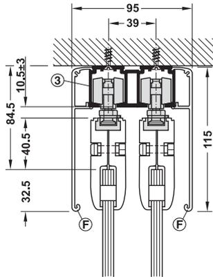
Ceiling installation with double running track and clip panel 115 mm
