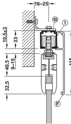
Wall mounting with mounting bracket and clip panel 115 mm
