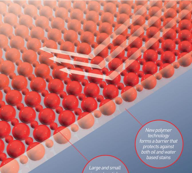
Large and small pigment particles embedded in the polymer reinforce the barrier
