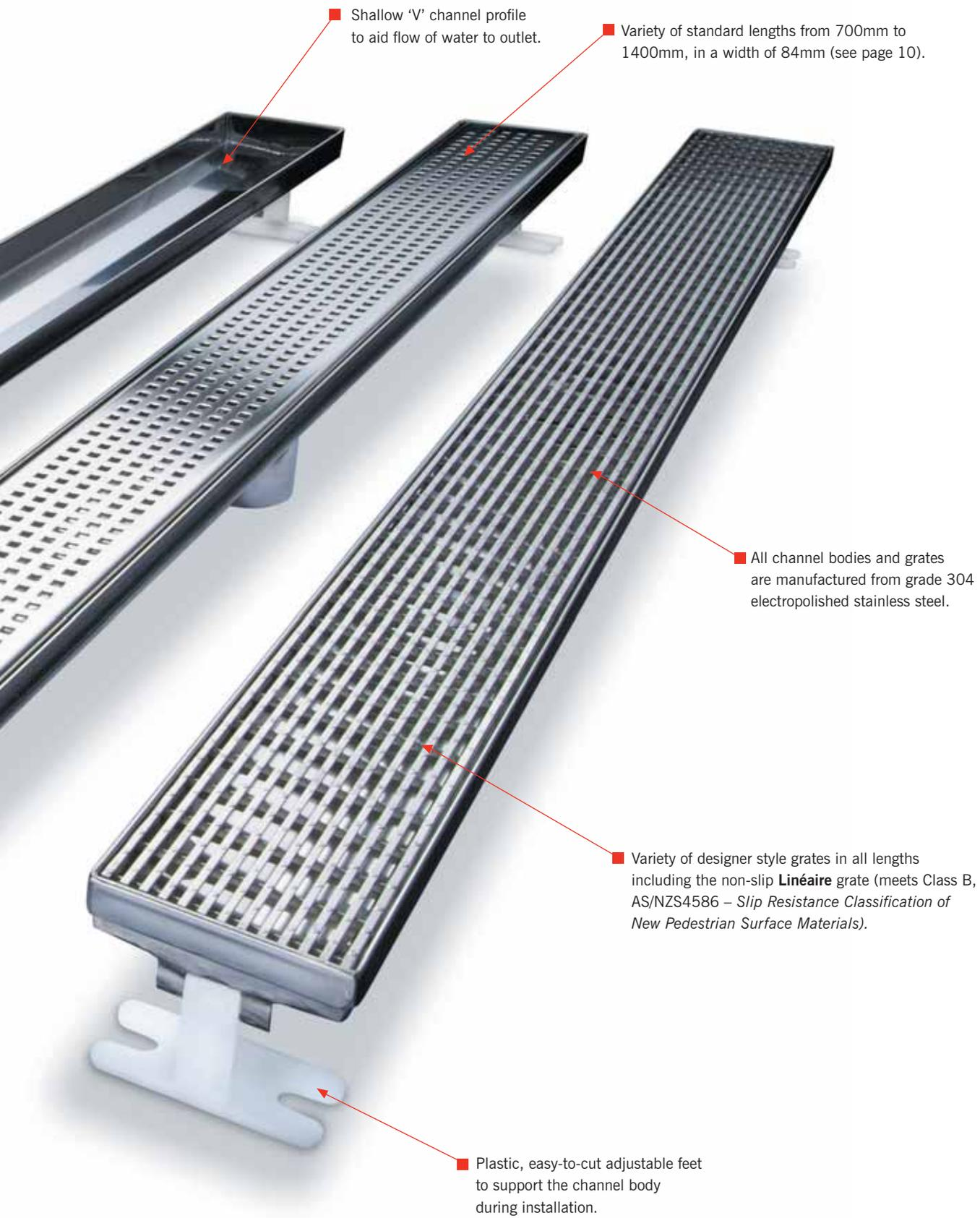
■ Shallow 'V' channel profile to aid flow of water to outlet.
