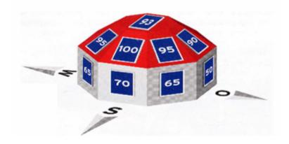
High energy yields are generated by arranging for the system to face south at a horizontal angle of 30° (100). The yield values will be somewhat lower if the direction deviates from this.
