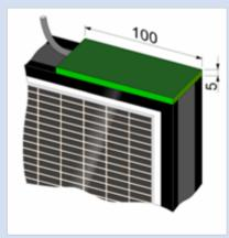
Cable outlet of a SCHOTT ASI<sup>®</sup> double glazing unit
