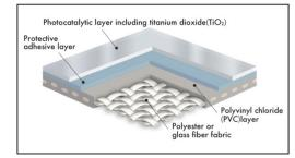
PVC-coated fabric with TiO2 is a combination of standard base cloth material coated in PVC, with TiO2 photocatalytic treatment added to the fabric surface. Due to the oxidation decomposition and highly hydrophilic nature caused by the TiO2, dirt can be easily washed off.
