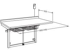
**Height-adjustable** from 650 – 1000 mm **Max. load R8711 - R8712:** 75 kg **Max. load R8713:** 150 kg
