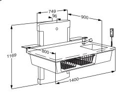
**Height-adjustable** from 300 – 1000 mm **Max. load R8682 - R8685:** 75 kg
