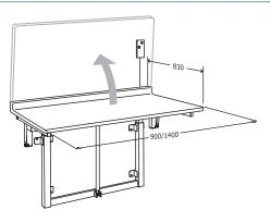
In raised position: 160 mm Height-adjustable from 650 – 1000 mm Max. load R8721 - R8722: 75 kg Max. load R8723: 150 kg
