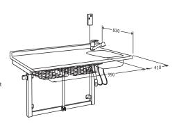
**Height-adjustable** from 650 – 1000 mm **Max. load R8732, R8734:** 75 kg **Max. load R8733, R8735:** 150 kg
