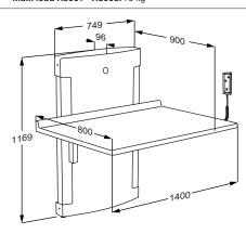
In raised position: 250 mm Height-adjustable from 300 – 1000 mm Max. load R8671 - R8673: 75 kg
