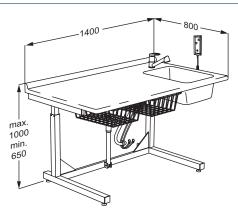
**Height-adjustable** from 650 – 1000 mm **Max. load R8652, R8654:** 75 kg
