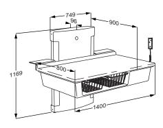
Height-adjustable from 300 – 1000 mm Max. load R8661 - R8663: 75 kg
