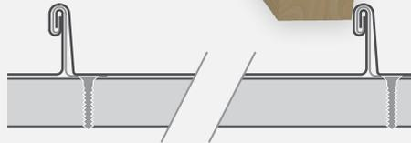
*Double lock standing seam profile and installation shown on 17mm ply board over supports.*
