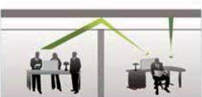
ULTIMA+™ dB ceilings provide an excellent level of **sound attenuation**. The product is ideal for spaces where privacy between rooms or where noise from above the suspended ceiling are important considerations.
