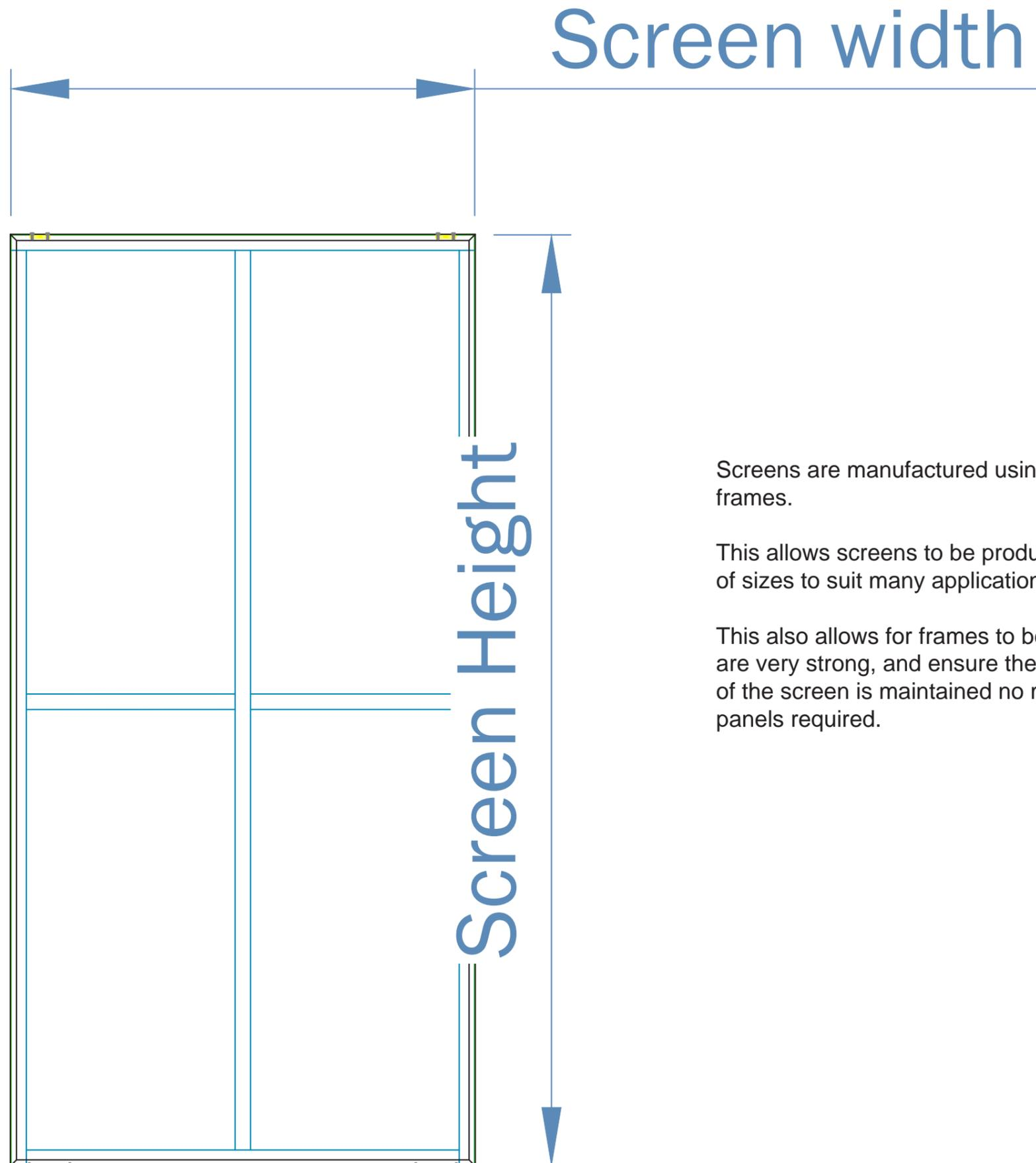
Screens are manufactured using aluminium welded frames.
