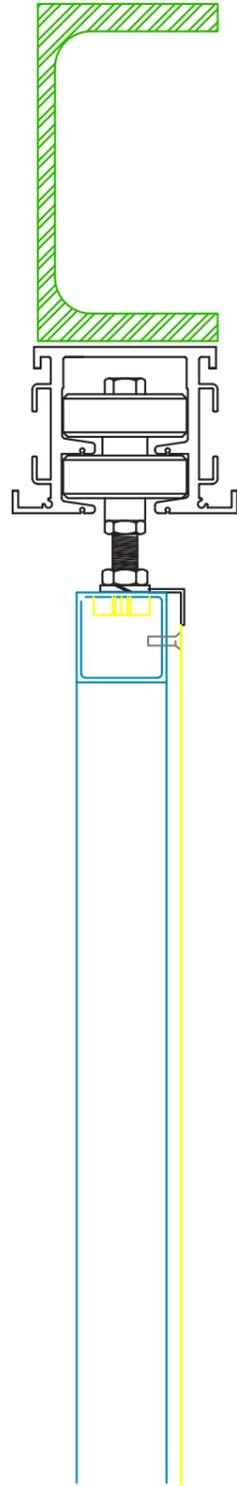
Multi Direction Track And Rollers for screens that can turn and stack in various locations. Tracks and Panels can be installed to create grids for use in projects such as Art Galleries
