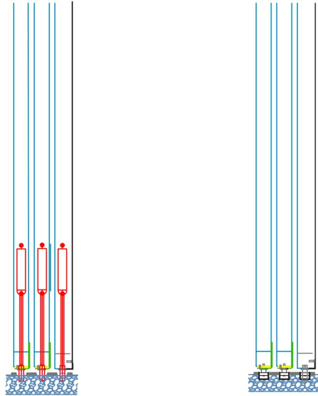
Screens can be installed with or without floor tracks and bottom floor guide rollers. Footbolts can be incorporated to lock panels in designated locations by use of flush finish ferrules.
