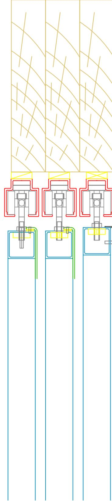
Linear track allow side by side track installation where screens move in two directions, independant of each other.
