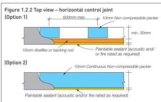
NOTE: Use 10mm wide by 16mm deep CSR Fireseal Sealant at vertical and horizontal control joints to achieve FRL of -/120/120 for the wall system. See Section 2.2. Protect Fireseal Sealant from rain until sealant has developed a thick skin. Once cured, Fireseal should be painted over with a compatible external grade acrylic coating i.e. Dulux AcraTex or similar.
