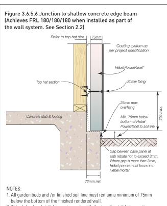
2. This slab edge detail does not comply with the termite visible inspection zone requirements. Alternate termite management systems must be used when selection this detail. It is the responsibility of the builder to provide a suitable physical or chemical barrier in accordance with AS 3660.
