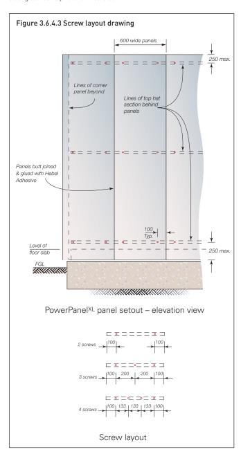
Figure 3.6.4.2 Hebel PowerPanel<sup>XL</sup> Zero Boundary Wall System fixing detail (Achieves FRL 90/90/90 when installed as part of the wall system. See Section 2.2)
