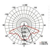
Luminous Flux Luminous Efficacy Output Power LED source Colour Temperature CRI 6206 lm 72 lm/w 86w 48 6500K >70
