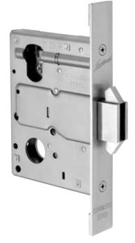
This series is available in a range of functions to suit sliding door applications. Locks are deadlocked by a cylinder and/or turnbutton. The deadbolt has claws fitted to the bolt which protrude or retract behind the strike.
