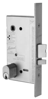
Combination locks are operated by handles/knobs from inside or outside. Both handles/knobs are locked by a cylinder and/or turnbutton. Lock automatically deadlatches when door is closed.
