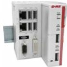
The ventilation controller processes all signals and information from the weather station, u::Lux buttons and the motor controller for effective and efficient ventilation.
