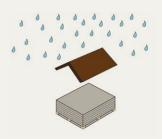
Protect boards from moisture and weathering before they are installed.
