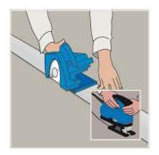
For sharp-edged cuts, for example, exterior edges, use a hand-held circular saw with a dust extractor or a pendulum jigsaw. Use of a carbide or diamond-tipped saw blade is recommended.
