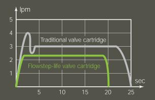
2) Filling a sink – Filling a sink or vessel with an over restricted tap can be frustrating, as it takes long to fill and does not save any water. With Pegasi, simply lift the handle to fully open for a good flow eg. 9lpm and get the job done. See diagram below. Based on Pegasi sink mixer with WELS 9lpm flow regulation versus other sink mixer with 6lpm flow regulator.
