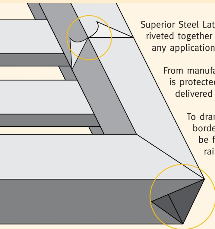
Superior Steel Lattice and Slatting is made from roll formed lattice strips, riveted together for strength and durability. It can be custom-made to any application and supplied either pre-fabricated or fully installed.
