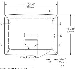
Rough Wall Opening 13-3/4" (350mm) wide 9-1/2" (240mm) high 3-3/4" (95mm) minimum recessed depth
