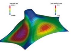
Higher stress concentration in weft direction. Note the different loads distribution on both directions of the membrane surface.
