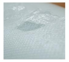
Image 1: "peeling effect" due to exaggerate lacquer thickness and bad adhesion.
