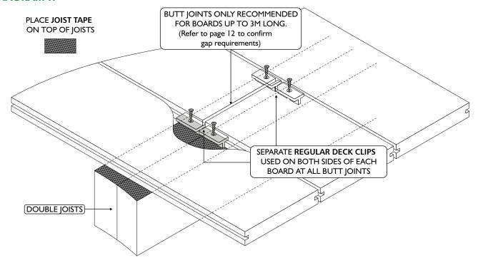
When fixing a butt joint use a Regular deck clip on both sides of each deck board (4 in total for each butt join, refer diagram H).
