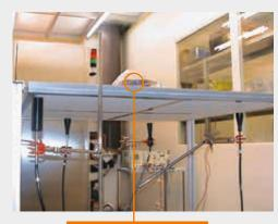
Reference loading through load speakers vibrations
