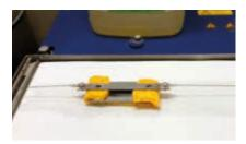
Scrubability tested according to modified ASTM D-2486
