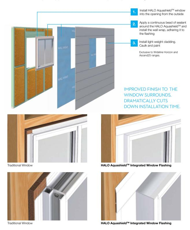
Halo Aquashield™ is a patented, innovative solution, designed to meet the requirements of modern building systems. It has been tested by NATA accredited testing laboratories and proven to provide higher water penetration resistance than traditional methods.
