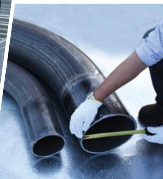
CNC Mandrel Bending is a highly specialised pipe bending process which gives the ability to produce tight radius bends with NO wrinkles or deformation.
