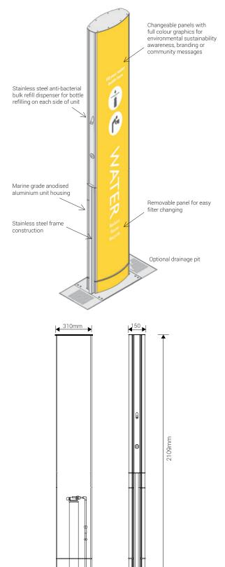
Front & side view with filter detail
