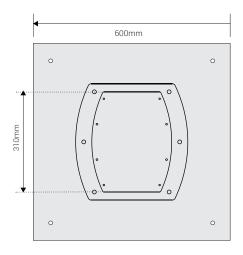
Plan view showing portable base plate
