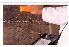
If the depth of the carbonation is known, then the rate at which it has occurred can be estimated for the year of construction. A cover metre will enable you to find the depth of cover over the reinforcing steel and therefore it is possible to calculate when the reinforcing steel itself will come under attack and expand through the overlaying concrete.
