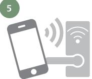
After ensuring that the Bluetooth is enabled, the guest simply holds the smartphone to the door lock, waits for the solid green light and enters the room.
