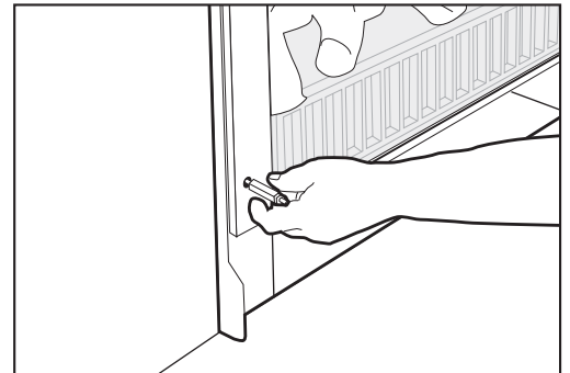
Figure (5) Remove four door studs used to secure the door.
