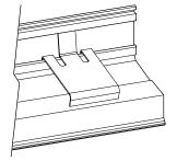
Step 2 Insert one small leg down into lower channel.
